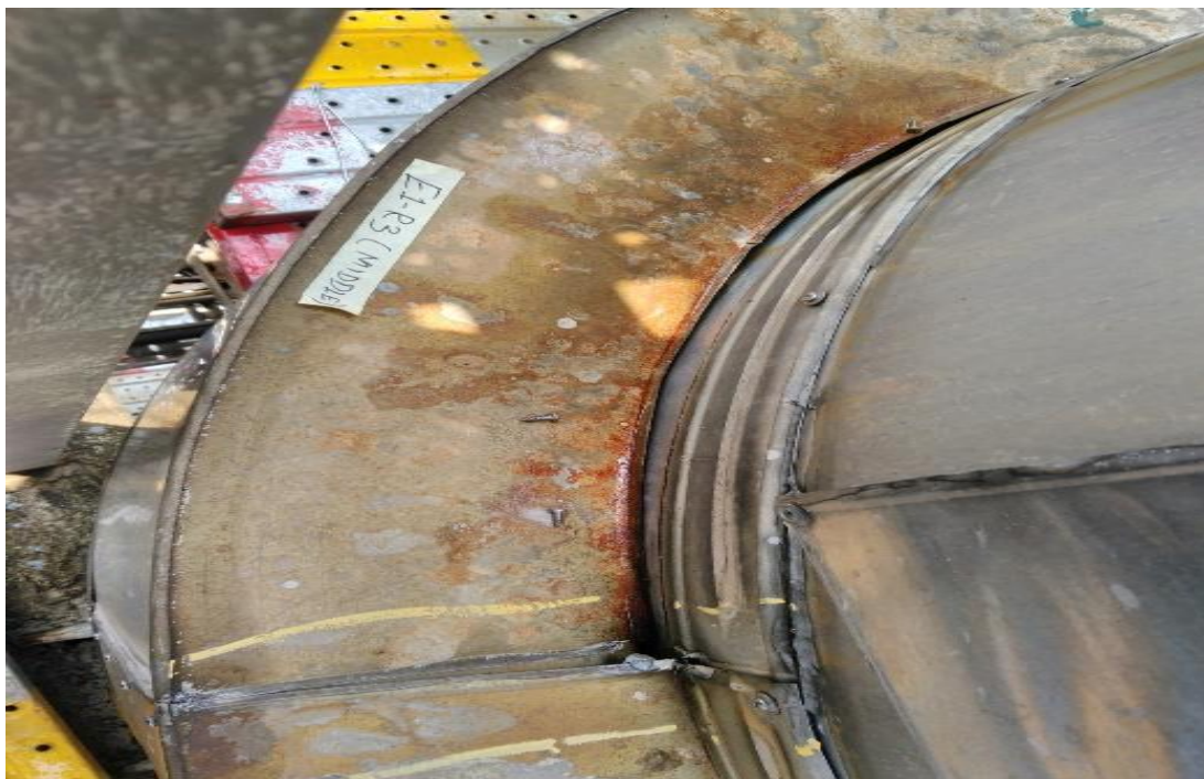
Photo 15: Flange attachment was in satisfactory condition
