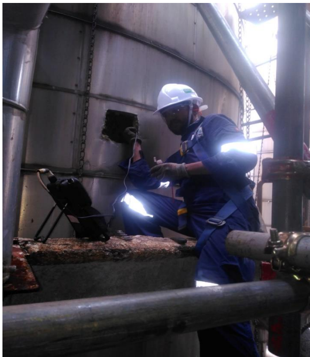
Photo 5: UTG measurement in Shell plates/ water jacket was done. External insulation was in satisfactory condition.
