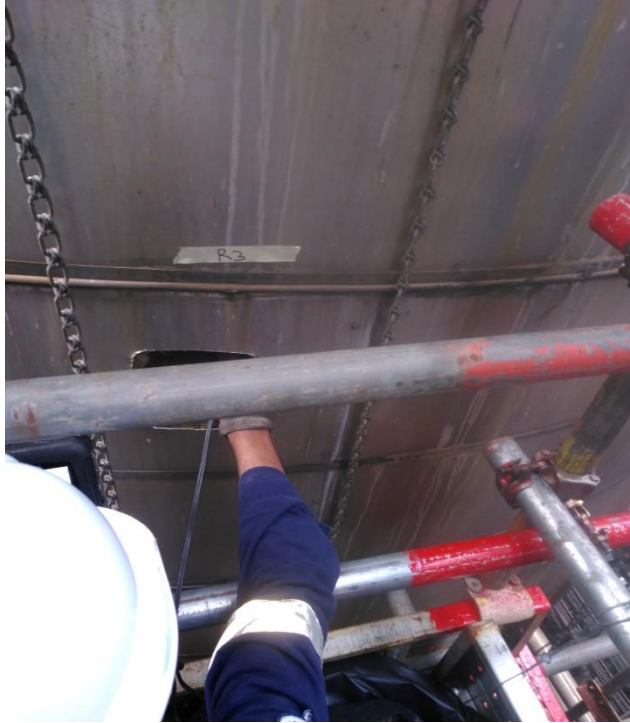
Photo 3: UTG measurement in Shell plates/ water jacket was done. External insulation was in satisfactory condition.
