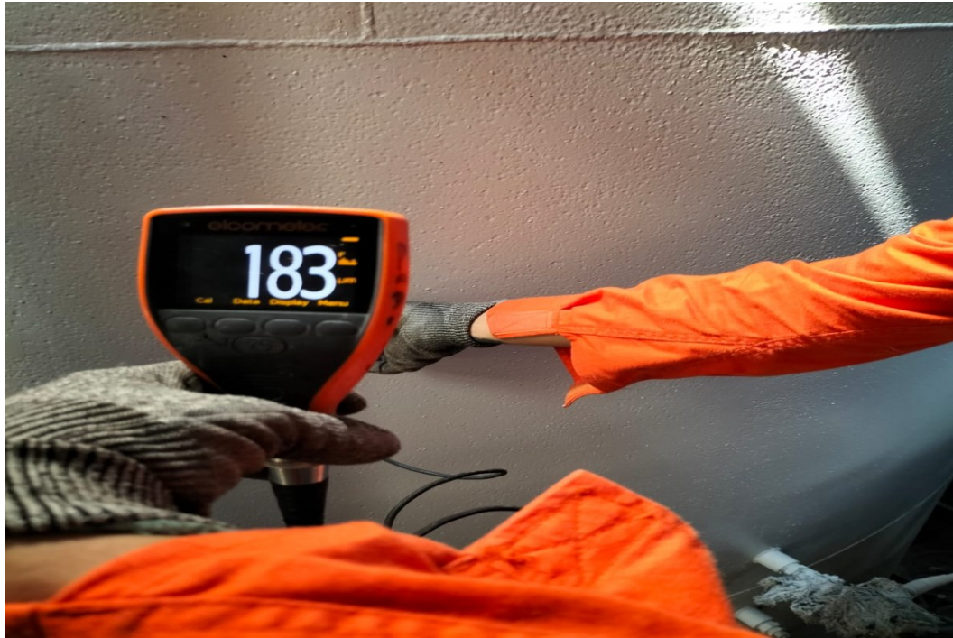
Photo11: Tank shell external was observed with general uniform pitting. Please refer to the pitting report for details of pit depth for each shell course. External coating (new) condition was satisfactory. Photograph showing after painting and DFT measurements.
