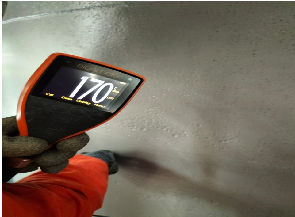
Photo 12: Tank shell external was observed with general uniform pitting. Please refer to the pitting report for details of pit depth for each shell course. External coating (new) condition was satisfactory. Photograph showing after painting and DFT measurements.
