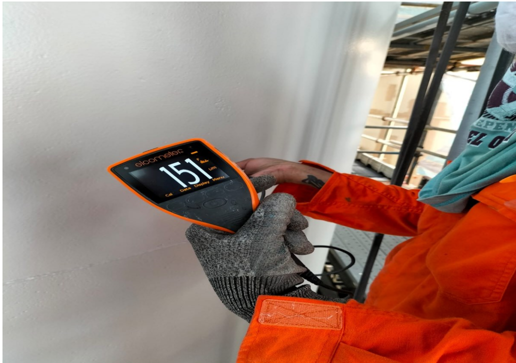
Photo 7: Tank shell external was observed with general uniform pitting. Please refer to the pitting report for details of pit depth for each shell course. External coating (new) condition was satisfactory. Photograph showing after painting and DFT measurements.
