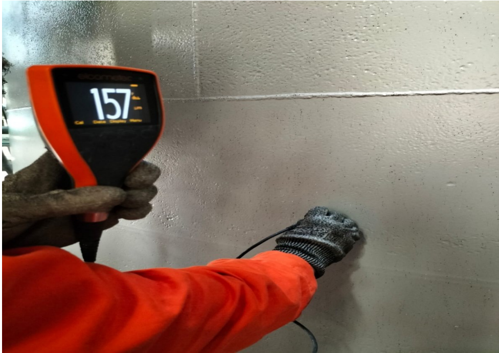
Photo 9: Tank shell external was observed with general uniform pitting. Please refer to the pitting report for details of pit depth for each shell course. External coating (new) condition was satisfactory. Photograph showing after painting and DFT measurements.
