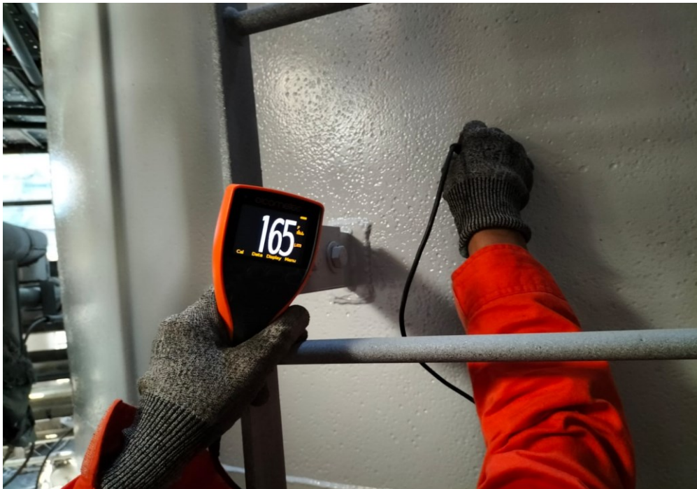
Photo 10: Tank shell external was observed with general uniform pitting. Please refer to the pitting report for details of pit depth for each shell course. External coating (new) condition was satisfactory. Photograph showing after painting and DFT measurements.
